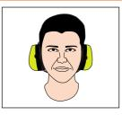
Adjust the length of the headband strap between the earcups so the earmuff fits well on top of the head. Place earcups over ears and make sure they fit snuggly to ensure equal pressure all round for comfort and max protection.
